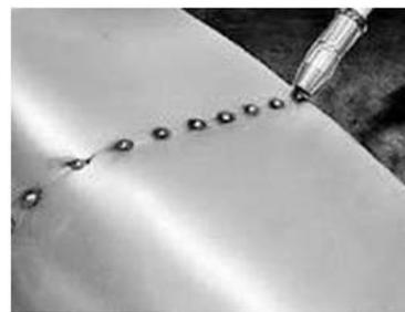
proceeding with the final weld. Both ends of each tack weld, representing start and stop (which are weak points often having unacceptable defects), must be ground to remove
