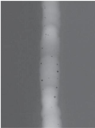
**Fig. 1** Porosity in a titanium weld
