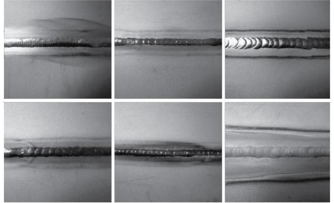
**Fig. 2** Varying levels of discoloration in Titanium weld
