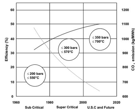
**Fig. 1.** Effect of operating conditions on efficiency and emissions of steam power plants.
