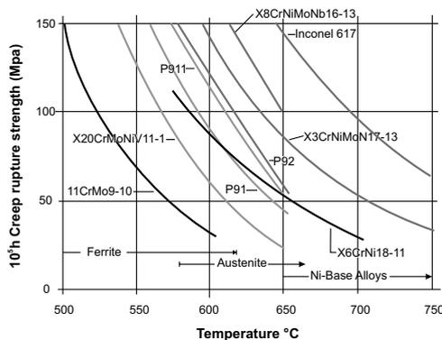
**Fig. 3.** Materials for main steam pipes in power plants
