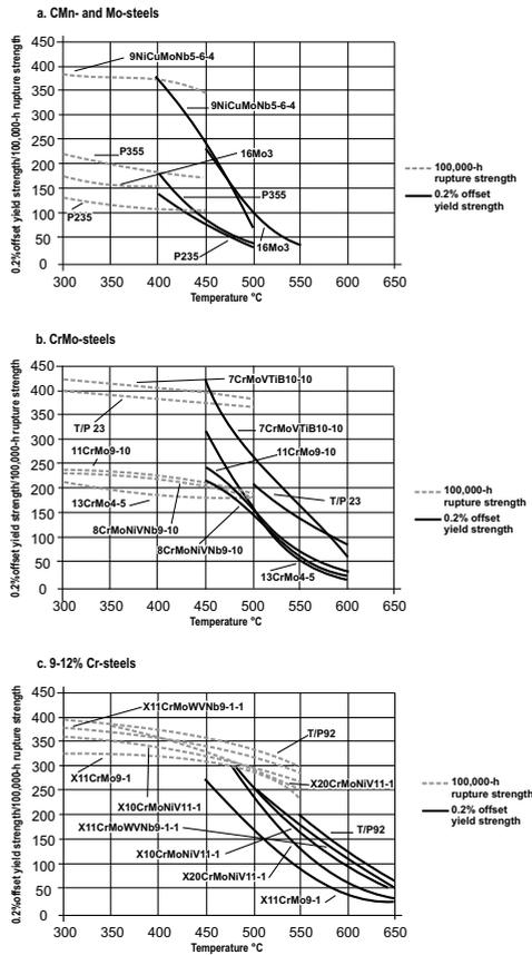
**Figure 2.** Creep-rupture strength of heat-resistant steels
