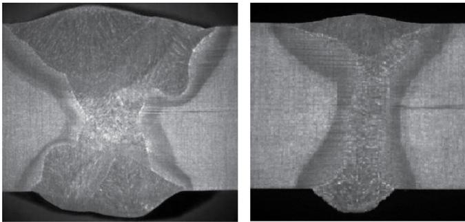
Fig. 1: GMAW weld vs HLAW weld on 12mm HSLA steel.
