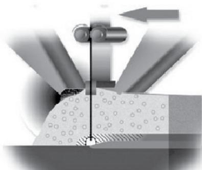
Fig. 1 Submerged Arc Welding
