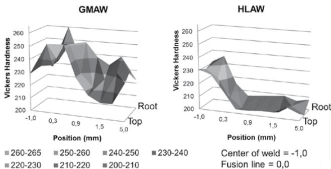
Figure 2: Micro-hardness measurements.
