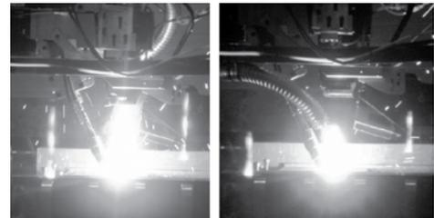
Figure 3: HLAW welding without (left) and with (right) plume management.
