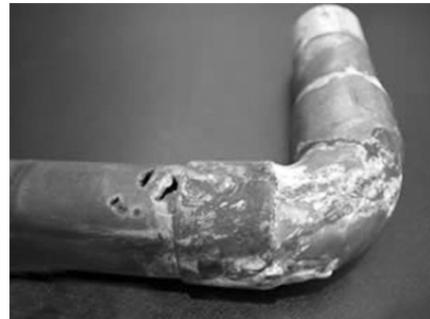
*Fig. 1 Corrosion of a copper-steel weld joint*
