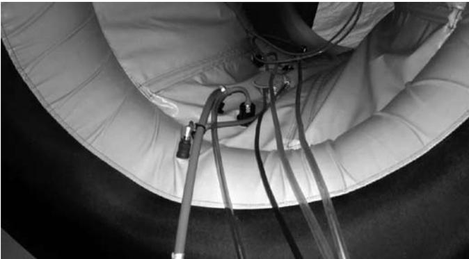
**Photo 2:** *Quick purge bladders with increase inlets and outlets*
