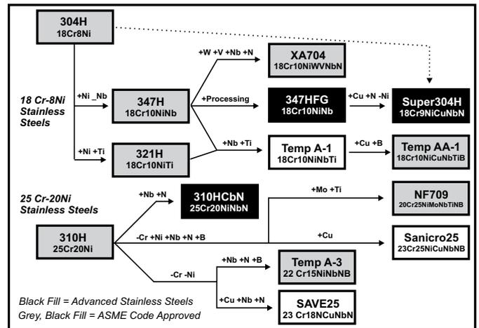
**Fig. 2** Process evolution of lean highly alloyed advanced Austenitic Steels
