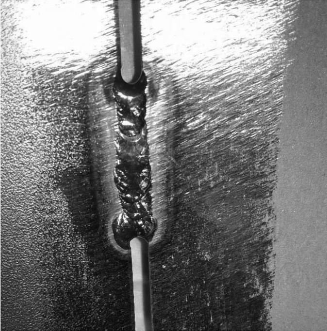
**Photo 1:** *Discoloured weld bead of titanium*
