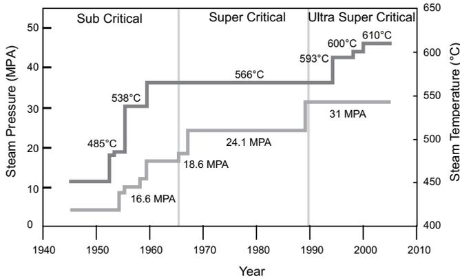
**Fig.1** Transition design of pressure and temperature in steam power plant
