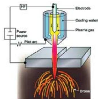
**Fig. 1** Schematic diagram of plasma cutting arrangement
