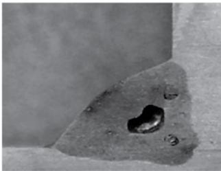
**Fig. 2.** Macroetch of fillet weld showing large irregular shaped porosity.
