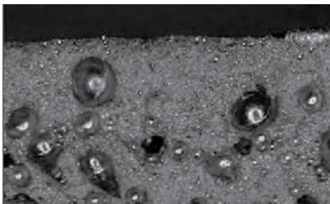
**Fig 3.** Scattered porosity in internal structure after nick-break testing.
