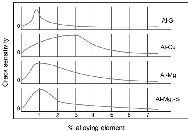
**Fig. 4.** Crack Sensitivity Curve
